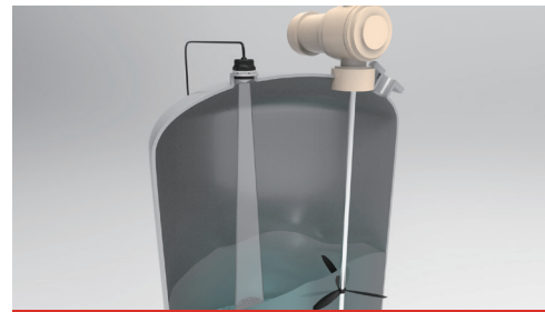
Open tank level measurement
